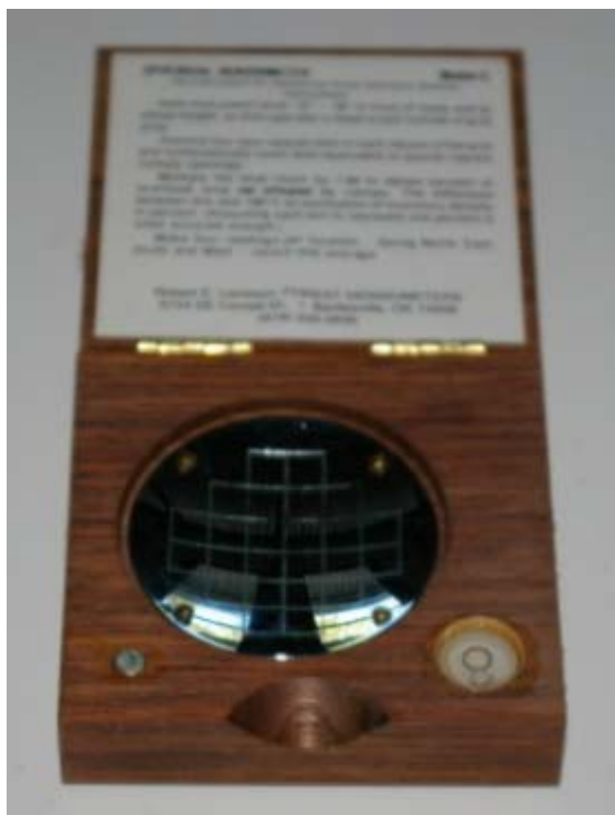
Fig. 2.8 – Concave spherical densiometer. The densiometer consists of a large, concave spherical mirror (center) with grids etched onto its surface. The smaller sphere in the lower right hand corner of the densiometer is a level used in taking densiometer readings. Each square in the grid is mentally subdivided by the user into four smaller squares. Light allowed through the overhead canopy is depicted as points of light on the mirror surface, with four possible points of light for each square of the grid. Visible points are summed, and this sum roughly estimates percentage of unobstructed canopy. The sum multiplied by 1.04 and subtracted from 100 provides the percentage of canopy density.
