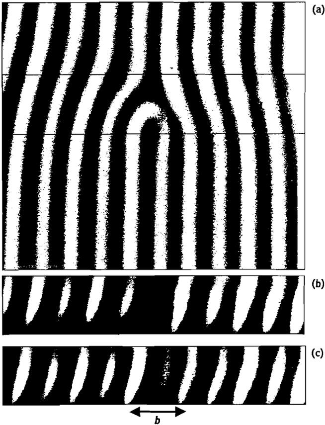
FIGURE 5.12. Confocal-microscope image of a dislocation  $b = p$  in the “fingerprint” cholesteric texture. The confocal microscope technique allows one to obtain the image of the director pattern not only (a) in the plane of the sample but (b), (c) in the vertical cross-section as well (photo D. Voloschenko).
