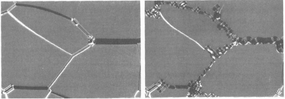
FIGURE 5.22. Network of oily streaks in a cholesteric planar texture. Cell thickness  $15\ \mu\text{m}$ , cholesteric pitch  $0.48\ \mu\text{m}$ . The oily streaks are (a) straight at zero voltage but (b) buckle when the voltage exceeds some threshold value. The short side of the field of view is  $420\ \mu\text{m}$ . The narrow streaks do not buckle while the wide streaks start to buckle at voltages higher than the medium width streaks.
