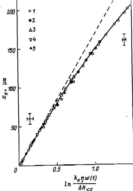
FIG. 2. Displacement of the layer of the photoinduced critical opalescence,  $x_0$ , under the influence of light for various values of  $\Delta T_{cr}$ : 1) 7.6; 2) 11.1; 3) 15.4; 4) 19.2; 5) 26.4°C. The dashed line shows Eq. (2) with  $K = K_0$ .
