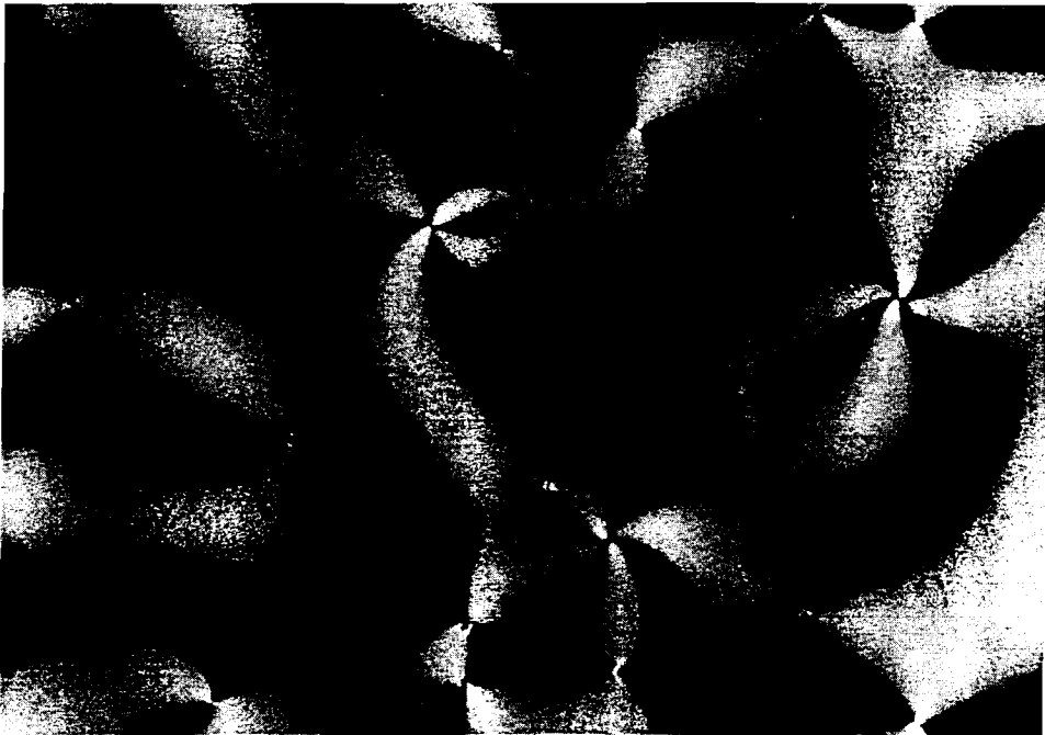
FIGURE 6 A typical Schlieren texture in a film of 4-pentyl-4'-cyanobiphenyl (thickness 23 \mu\text{m} ) between two glass plates coated with thin layers of glycerol.
