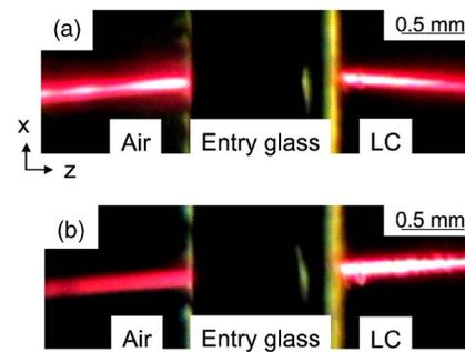
FIG. 4. (Color online) Photographs of voltage-controlled amphoteric refraction of a laser beam linearly polarized in the plane of figure, on passing through air into the entry glass plate,  $\theta_i \approx 5.5^\circ$ , and then into the LC. At zero voltage, refraction is negative,  $\theta_{r,S} \approx -4.2^\circ$  (a); at  $U=5$  V, it switches into the positive one,  $\theta_r \approx 3.8^\circ$  (b).
