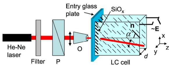
FIG. 3. (Color online) Experimental setup. The  $\text{SiO}_x$  coated glass plate is the entry plate for the laser beam. At zero voltage, the director  $\mathbf{n}$  is in the  $x$ - $z$  plane. The electric field  $\mathbf{E}$  serves to reorient  $\mathbf{n}$  along the  $y$  axis.
