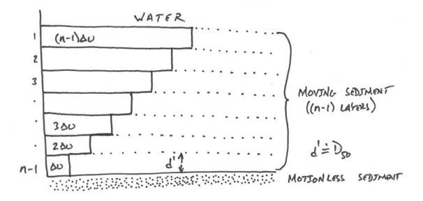
The bed moves as a series of superimposed layers of thickness d' (about the same thickness as D<sub>50</sub>). The velocity increases linearly (near the bed). If the  $(n-1)^{st}$  layer from the top just begins to move at velocity  $\Delta u$ , the  $(n-2)^{nd}$  layer (which is moved at  $\Delta u$  with respect to the  $(n-1)^{st}$  layer) is moving at  $2\Delta u$ . Extended up to the surface, the layer moves at (n-1)  $\Delta u$ . The total discharge / unit width =  $\overline{u}nd'$ .
