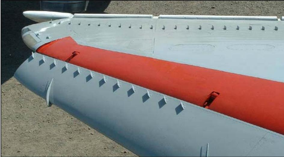
It turns out the little fins are called *vortex generators*, and their whole job in life is to force the boundary layer on the wing to become turbulent. Why would you want to do that? Turbulence increases drag, right?
