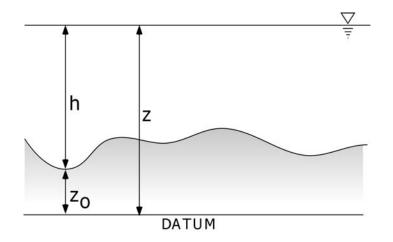
At this point, we could *define* a component of the total head that only contains the flow depth and the velocity head.
