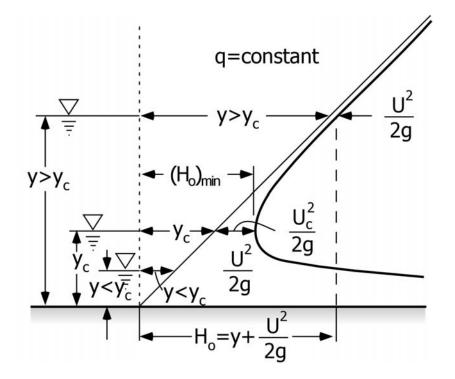
Notice what this is saying—there's one flow depth where most of the specific head is held as potential energy (h), and just a little is held as kinetic energy ( $U^2/2g$ ), AND there's one where most of the energy is kinetic, and little is potential.
