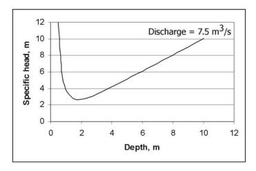
Because this graph has the shape of a parabola (in part), it says that above some critical depth, there are *two* permissible flow depths that will yield an identical discharge. Let's take a look at this where flow depth is actually on the vertical axis like we'd expect:
