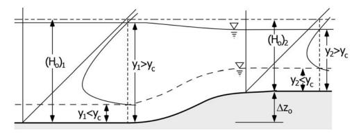
Above the critical depth (F=1), flow responds to a decrease in specific head by increasing the velocity and decreasing the flow depth. *Below* the critical depth, flow responds to a decrease in specific head by decreasing the velocity and increasing the flow depth. Flow deeper than F=1 is called *subcritical* or *streaming* flow.
