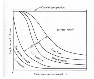
Remember it? It shows early rain being intercepted by trees and the like, and a lot of rain filling up depressions in the watershed. Also, it shows that Hortonian curve—water infiltrating quite a bit at first, and then tailing off. Eventually, then, most of the rainfall becomes runoff, which in turn affects our hydrograph. I'd like to spend today talking about hydrographs and what affects them.
