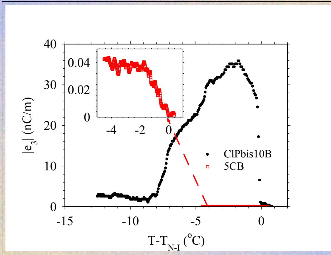
*Variation of the flexoelectric coefficient on a relative temperature scale  $T-T_{N-I}$  for the bent-core liquid crystal ClPbis10BB as well as for the calamitic liquid crystal 5CB measured in cells of  $A=1\text{cm}^2$  active areas. The inset shows part of the figure ( $|e_3|$  of 5CB) at a magnified scale.*
