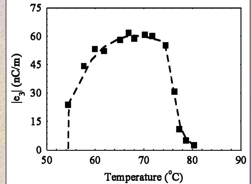
*Displacement dependence of flexoelectric current (in rms values) of ClPbis10BB at 74 $^{\circ}$ C; (b) the temperature dependence of  $|e_3|$  of a well aligned cell measured at 5Hz in 15mm x 15 mm active area plastic cells*
