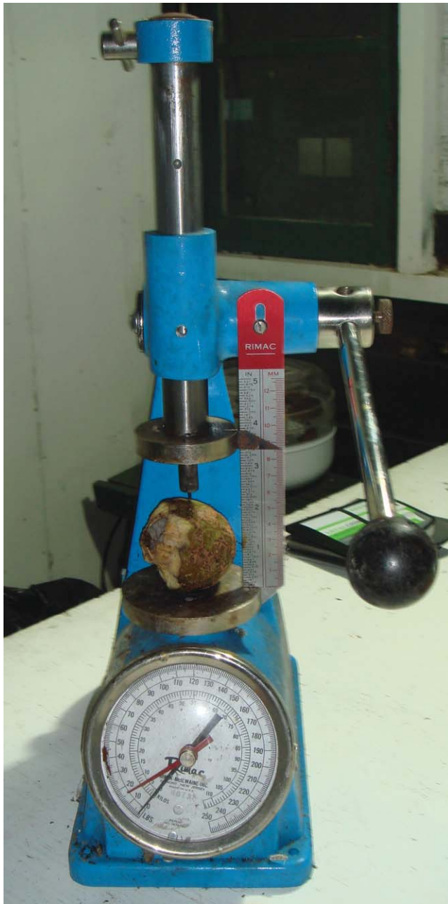
Fig. 5. Rimac spring tester fitted with a 1.6 mm diameter pin to test puncture resistance of fruit >10 kg/mm 2 . Tontelea coriacea (Celastraceae) partially eaten by Pithecia pithecia is pictured. [Photo by M. Norconk].
