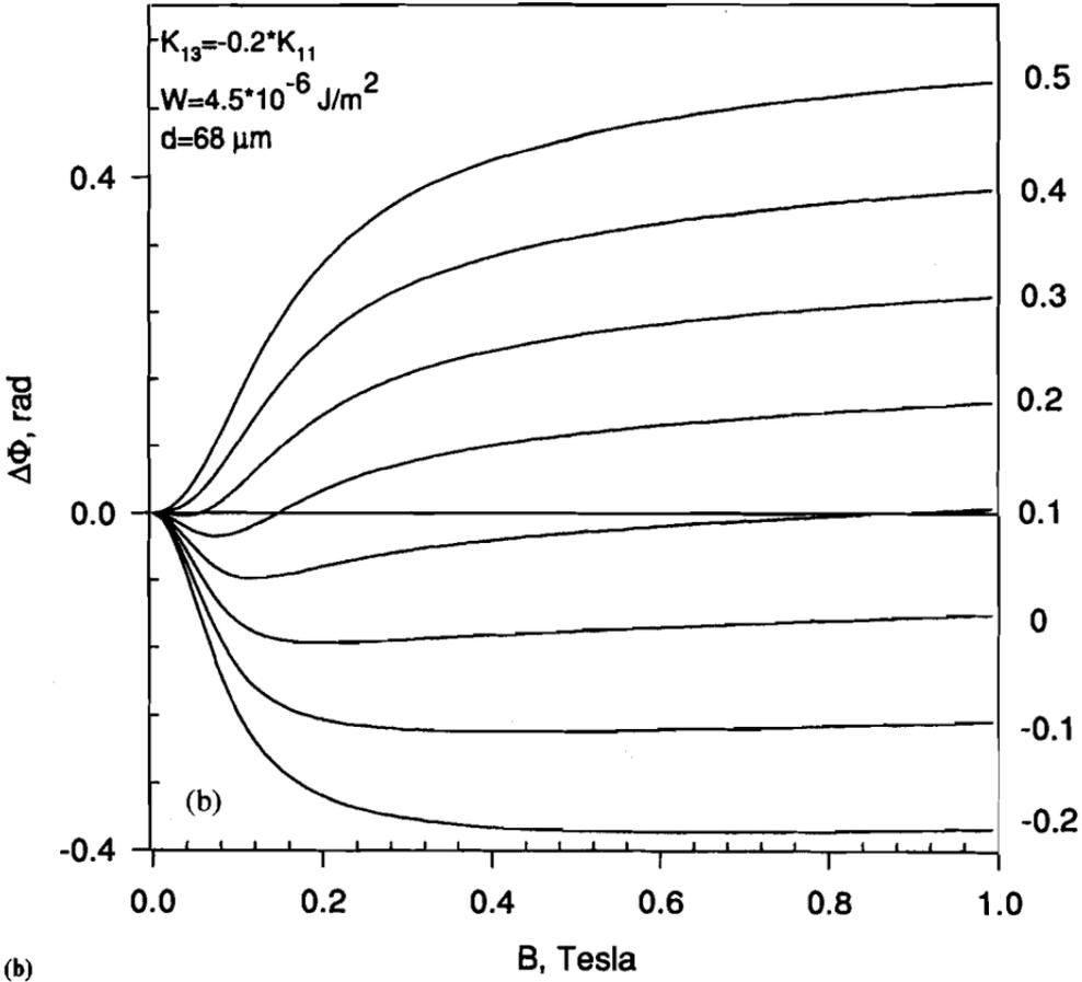
FIGURE 2 Phase retardation as a function of the magnetic field and the angle  $\bar{\psi} = \bar{\theta} - \alpha$  (shown in degrees on the right side) for  $K_{13} = 0$  (a) and  $K_{13} = -0.2 K_{11}$  (b); other parameters are indicated in the text.
