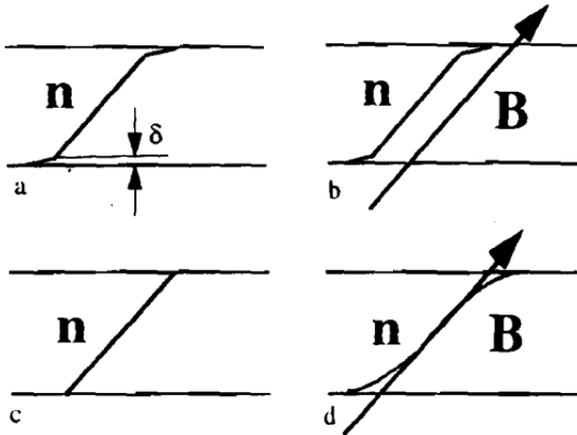
FIGURE 1 A nematic cell with tilted boundary conditions in zero (a,c) and non-zero (b,d) magnetic field applied parallel to the easy axis. Director distribution is shown schematically as predicted by the theory with strong molecular deformations (a,b) and by the first-order theory (c,d). The scale of deformation  $\delta$  in (a) is molecular; the scale of deformations in (d) is macroscopic.
