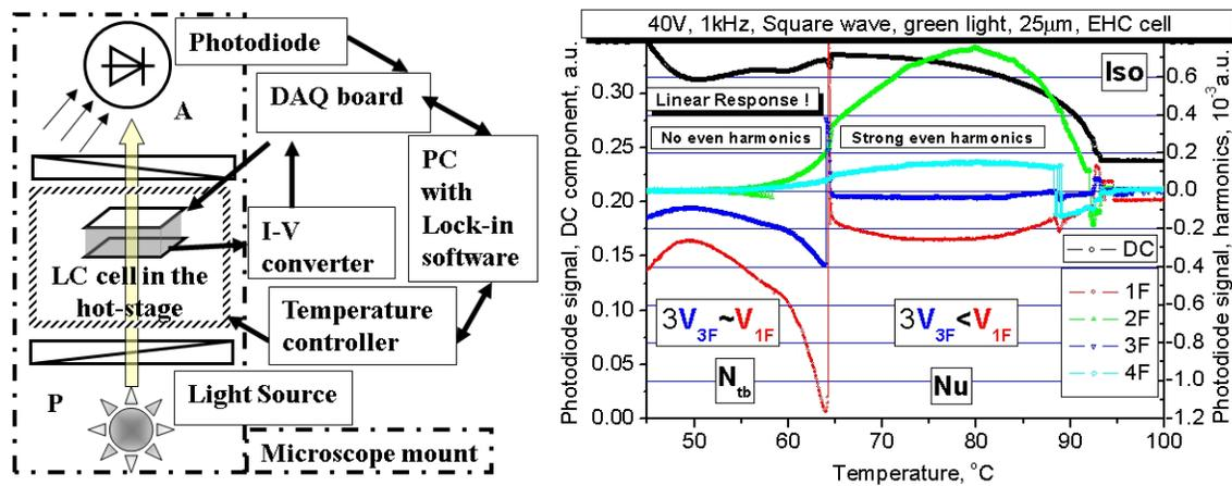
Figure 3. Left: the optical contrast spectroscopy set-up. Right: Temperature dependence of the various harmonics of the optical response.
