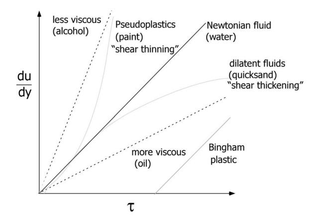
For a Newtonian fluid, the slope of the line is a measure of how efficient the fluid is at transmitting velocity. The flatter the slope (on these axes), the more efficient the fluid is at transmitting velocity downward.
