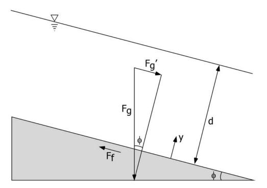
This is just like the torque converter, except that there's no plate on top! No plate means no stress, so at the top of the flow  $\tau=0$ . At the *base* of the flow, though, the stress is exactly balanced by the force of gravity acting downslope. The gravity part is easy:
