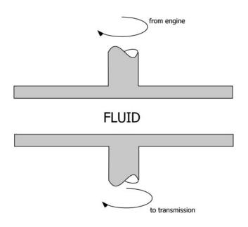
What's happening is that as molecules of transmission fluid slide along the bottom, or even slide past each other, some of their energy of motion is dissipated as heat. Picture the fluid gap as very very thin slices of fluid:
