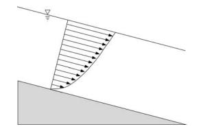
This is what happens if viscous forces are the only ones involved in the problem; it works for a relatively viscous fluid (like ice, or transmission fluid) on a perfectly smooth bottom. For a rough bottom, however, we get flow separation and non-parallel stream lines, so:
