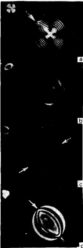
FIG. 1. CLC drop with  $R = 35 \mu\text{m}$  in glycerine. The nichols are crossed. a) Monopole structure with  $\chi(+2)$  line,  $P = 6.5 \mu\text{m}$ ; b, c, d) show the degeneration of the  $\chi(+2)$  line into two singular points and their divergence toward the poles of the drop ( $P \approx 40, 60 > 100 \mu\text{m}$ , respectively). The defects are indicated with arrows.
