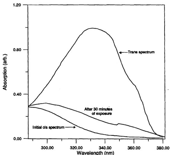
FIGURE 3 The absorption spectra of 7AB polymethylmetacrylate: relaxation of the initial spectrum of predominantly *cis*-7AB (*UV*-irradiated) under He-Ne irradiation at room temperature.
