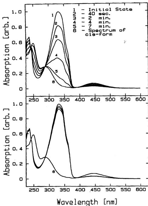
FIGURE 2 The absorption spectra of 7AB in octane. Initial states in are close to the pure transform; (a) transformation of the initial spectrum under *UV* irradiation by a 366 nm source; (b) transformation of the spectrum 1 under irradiation by a 437 nm source.
