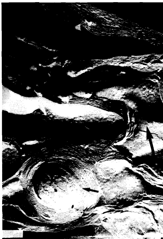
Fig. 4. — Freeze-fractured specimen, electron microscopy observation : in the middle of the L_\alpha phase. Note the presence of spherulite embedded in the lamellar phase. The lamellar phase shows positive Gaussian curvature (small arrow) as well as negative Gaussian curvature (big arrow). \text{hex/CpCl} = 0.8 ; 85 % solvent. Bar 0.5 \mu\text{m} .
